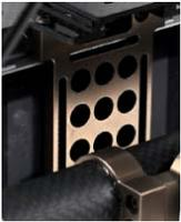
The metal spacing board which is the back of the camera frame could be adjusted for balancing the camera gravity when use a different lens. After the adjustment, lock the 4 screws ( 2 on the top and 2 under the bottom ), next time just push the camera to the metal spacing board, that is the center of gravity.
